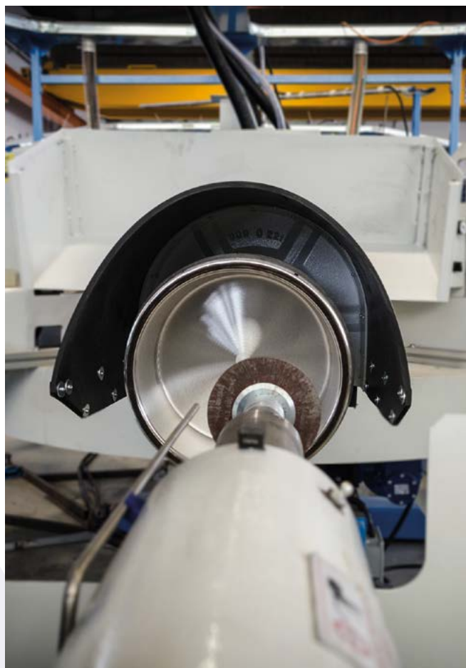
Smerigliatura parete interna pentole - Internal wall grinding for pots
