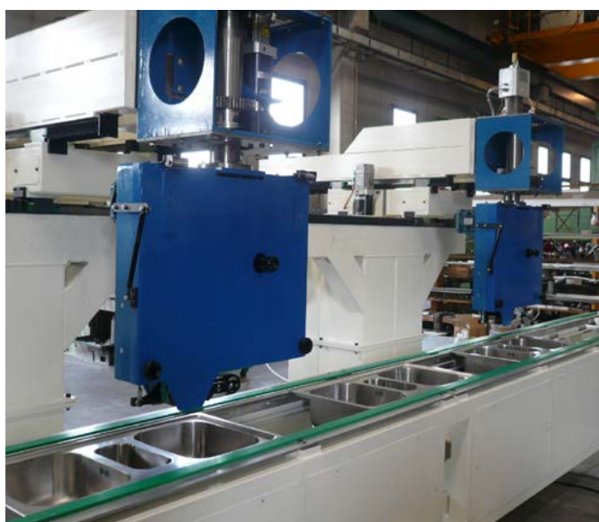
Transfer smerigliatura - Transfer grinding system
